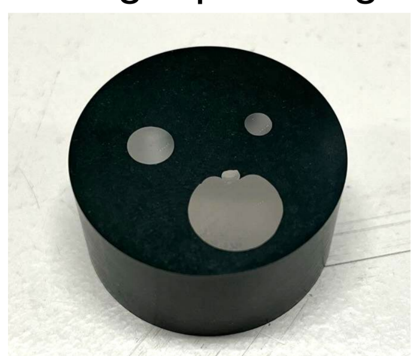
Fig. 2: Mounted and polished heat treated samples
