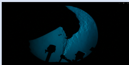
Figure 2: Raw Footage of Gas Leak recorded by Schlieren
